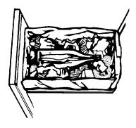
Bottles or cans not placed in the centre may become caught between the ram and the drawer. The Drawer Monitor Switch senses a "misload" and causes the ram to return to the "up" position without compacting. Load bulky trash, bottles and cans in the **centre** of the drawer.
